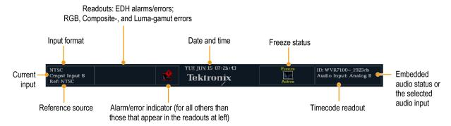
Figure 1: Status bar in single input mode
