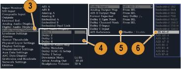
Select Format Expected and choose the format condition that, when missing, triggers the Dolby Format Alarm.
