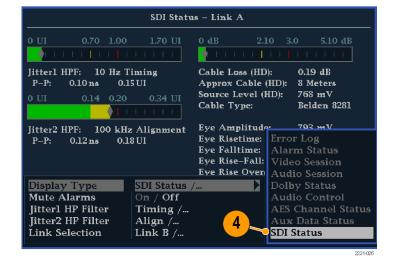
Use the Cable Loss thermometer and readouts to monitor the cable loss.
