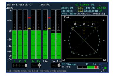
16. Select Downmix Mode. Each downmix mode combines multiple separate audio channels into a mix that provides compatibility for users with only mono or stereo systems, or with older analog surround sound systems.
