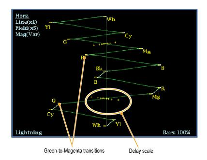
The + tic marks on the graticule indicate the following timing errors:
