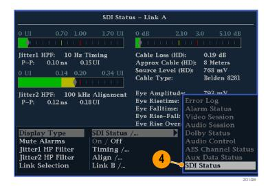
**5.** Note the Eye waveform measurements in the SDI Status display readouts.
