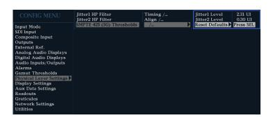
Select Jitter1 Level. Use the General knob to increase or decrease the threshold level for the Jitter1 engine controlling the top two tiles of the instrument display.
