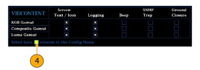
Check that Enable Alarms is set to On in the Alarms menu before leaving the Alarms menu.
