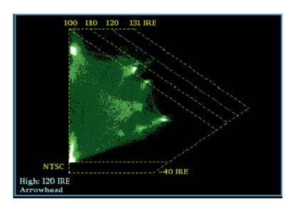
Another useful Arrowhead function is a measure of how well the active video signal is using the dynamic range of the video channel. A properly adjusted signal should be centered in the arrowhead graticule and have transitions that approach all the limits.
