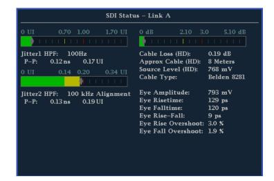
Automatic Eye measurements (and a histogram of the Eye waveform) are also displayed in the Eye Waveform display when expanded to the single, full-screen display.
